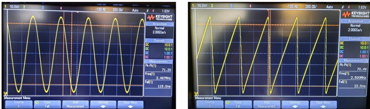
Figure 21: Screenshots from the testing of the driver unit of Figure 20. (Left): Output signal with 71.2 Vpp in the case of sinusoidal input at 2.5 MHz. (Right): Output signal with 70.4 Vpp in the case of a sawtooth input signal at 2.5 MHz.
