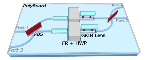
Figure 1. Schematic layout of the four-port optical circulator. It consists of two polarization beam splitters/combiners (PBSs) and two Faraday rotators and half wave plates (HWPs) integrated via an on-chip collimated beam section created by two pairs of waveguide coupled GRIN lenses and passive polymer waveguides (dark blue).
