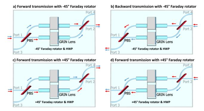
Figure 2. Working principle of the optical circulator in forward and backward transmission for TE (red arrows) and TM (blue arrows) polarized light with a  $-45^{\circ}$  Faraday rotator (a, b) and a  $+45^{\circ}$  Faraday rotator (c,d). The output port depends on the magnetization and direction of Faraday rotation of the Faraday rotator.
