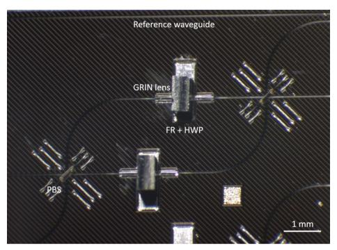
Figure 3. Optical circulator, consisting of polymer embedded single mode waveguides, PBSs, HWPs and Faraday rotators that are inserted via on-chip free-space sections created by waveguide coupled GRIN lenses. The fabricated device has length of 9 mm and a width of 7 mm.
