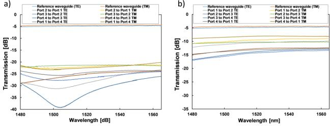
Figure 4. Measured insertion loss, including fiber-chip coupling losses of ~1.5 dB per facet, in forward (a) and backward (b) transmission for all ports in TE and TM polarization.
