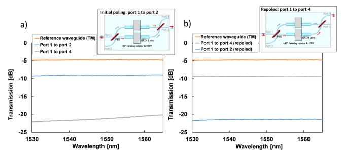
Figure 5. Repoling between the ports enables switching as illustrated in Figure 2 (a) and (c). Here, switching is demonstrated for port 1 as the input port and port 2 and 4 as the output ports. a) Initial poling with transmission from port 1 to port 2 and optical isolation of port 4. b) Repoled Faraday rotators with transmission from port 1 to port 4 and optical isolation of port 2.
