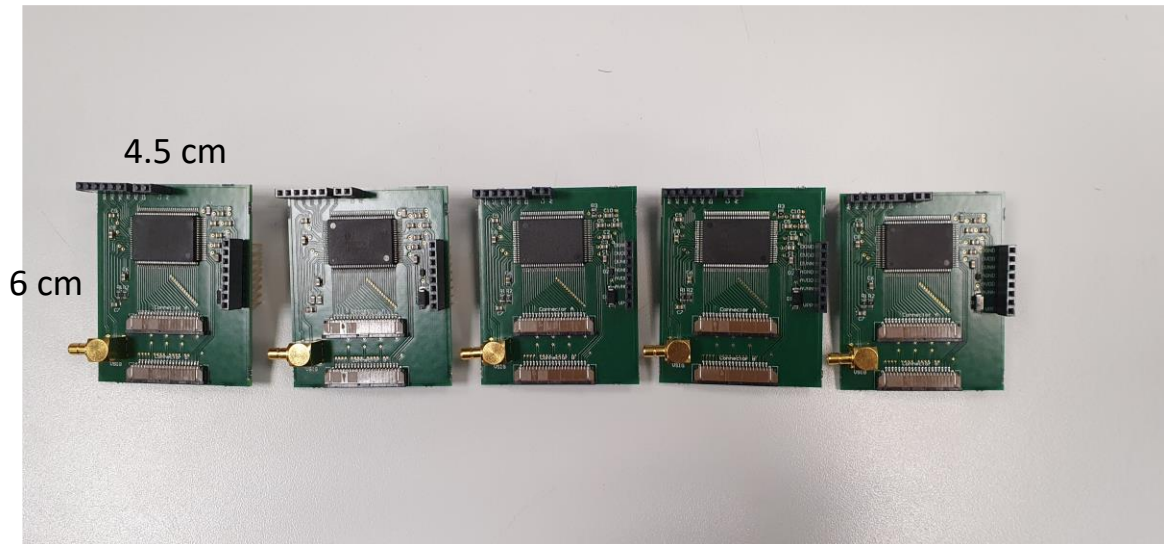
Figure 14. 32-channel High-voltage, low-speed driving circuits
