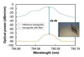
Fig. 4: Transmission through a waveguide with TFF for the suppression of 785 nm light compared to a reference waveguide without filter. The inset shows an exemplary PIC with inserted dielectric TFF.
