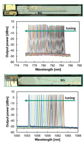
**Fig. 1:** Emission spectra of hybrid tunable lasers at 785 nm (top) and 1064 nm (bottom). The color-coded emission lines correspond to different operating points of the lasers. The microscope images show the hybrid integrated lasers consisting of GaAs-based gain chips (GC) and polymer-based Bragg gratings (BG).
