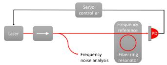
Fig. 2. Setup with feedback loop for frequency stabilization of the hybrid-integrated laser. The setup contains the laser, an isolator  $(\rightarrow)$ , a fiber loop that serves as frequency discriminator, a photodiode (PD) and a servo controller.
