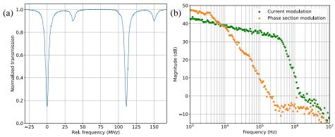
Fig. 3. (a) Normalized transmission through the fiber ring resonator, recorded by scanning the laser current. (b) Magnitude response for modulating the amplifier current and phase section of the laser.
