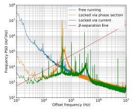
Fig. 4. Recorded frequency-noise power-spectral-density (PSD) for the free-running laser in comparison with the frequency-stabilized laser. Feedback is applied both to the amplifier current and the phase section.
