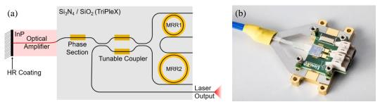
Fig. 1. (a) Schematic view of the hybrid-integrated laser. Heaters for thermal tuning of the laser are indicated in yellow. (b) Photograph of the hybrid laser assembly. Photo by Gijs van Ouwerkerk, PHIX Photonics Assembly.
